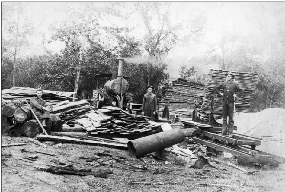
This view of a portable sawmill in the timber features a steam tractor-driven circular saw with logs and stacks of sawn lumber. The Gill Collection (see sidebar at right) contains a similar sawmill producing railroad ties.
